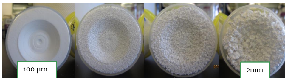
Figure 3. Powder and granules of BG with particle size ranging from <100 \mu\text{m} to 2mm.
