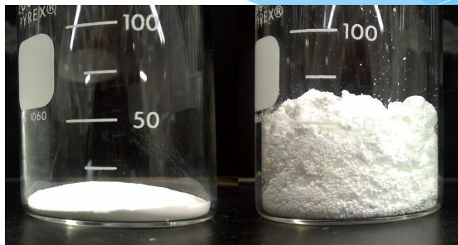
Figure 6. Corn starch before (left) and after PGX processing (right), showing the same mass of corn starch in both containers.
